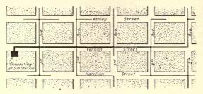
Fig. 145.—Showing a tree circuit as applied to out-of-door distribution. (This type of a circuit is called a "tree circuit" because of its resemblance to the trunk and branches of a tree.)
